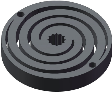
Figure 9.4: Symmetric torsion spring from strong-yet-malleable maraging steel, where the reaction forces of both windings are canceled out, keeping spring center always in the middle.
