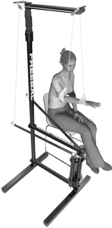
Figure 4.2: The Freebal. The system generates the weight supporting forces with almost inertia-free ideal-spring mechanisms (see Fig. 4.3). The wrist and elbow are supported by two slings connected via cabling to these independent mechanisms. In the figure, the overhanging beam is shown lowered for display reasons. During normal use, it can extend up to 3.5 m above ground level dependent on available space and the work volume needed.
