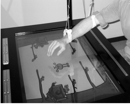
Figure 5.1: Training setup with FurballHunt game. In the game, the user has to chase away little birds called Furballs which fly from a birdhouse to one of the tree branches. The bird can be chased away by touching it with the hand, as detected by capturing software. The suspension slings from the Freebal (see Chap. 4) are visible at the wrist and elbow.
